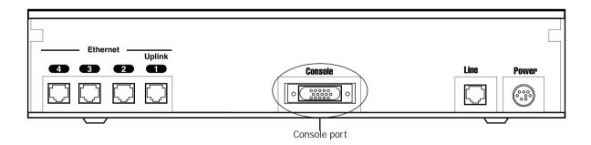
To connect the Netopia R310 to your computer for serial console communication, use the supplied dual console cable connector end appropriate to your platform:
